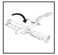
Lift the baseplate locking leaver and rotate the vertical arm down onto the baseplate.
