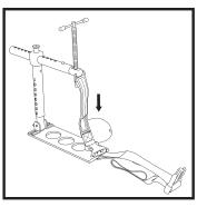
To store the CRoC in the combat ready configuration, remove the pressure disc.
