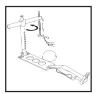
Depress the vertical arm locking pin and rotate the horizontal arm 90 degrees.
